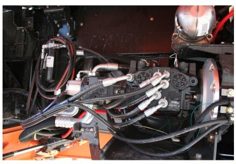
双液压泵提供左右两套驱动马达 Twin Hydraulic Pumps provide hydraulic flow to right and left drive motors
